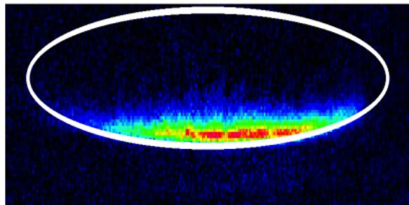
Atoms are confined to the isopotentials of a quadrupole field.
