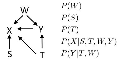
$$P(X,Y,W,S,T) = P(X|S,T,W,Y)P(Y|T,W)P(W)P(S)P(T)$$
