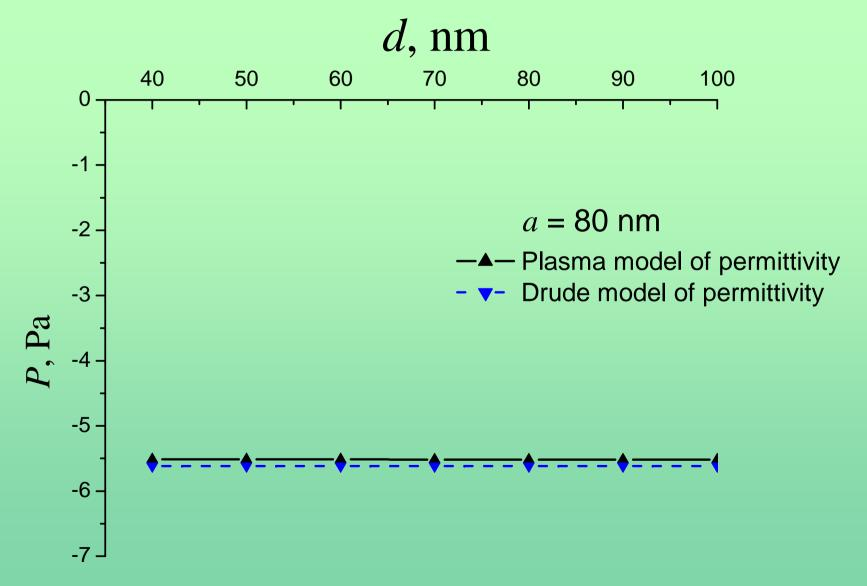
**2.** Calculated dependence of the Casimir pressure on the thickness of the layer with increased carrier concentration.
