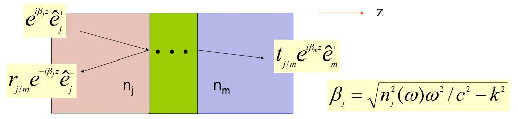
Note that  $r_{j/m}$ ,  $t_{j/m}$ ,  $r_{m/j}$  and  $t_{m/j}$  are Fresnel coefficients of a planar object (a stack of layers) between two semi-infinite local layers j and m (that is, of the system j...m denoted shortly as j/m).
