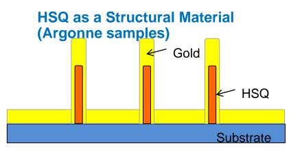
Inorganic negative tone e-beam resist Minimum feature size: ~6nm High aspect ratio lithography: ~10:1 (380nm tall, 40nm wide)
