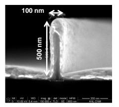
Sputtered gold deposition (Kurt Lesker PVD Sputter/E-beam) 120nm Au / 20nm Ti (~130nm actual thickness)
