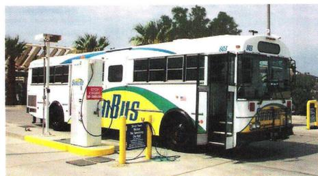
A SunLine Transit Agency "SunBus" with Cummins Westport 5.9-litre B Gas Plus engine, refueling with HCNG. Also shown is the HCNG dispenser.
